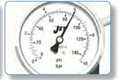
STEP 6. If all remains well, reduce pressure to operating pressure. For screeded floors, pipework should be left to approxiamately 3-6 bar until the screed has been laid and dried to protect pipework from damage. Consult screed supplier for drying out and curing time.
