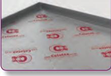
**STEP 2.** Floor panels should be fitted to a suitable flat sub base. Extra insulation maybe required to match design or building regulations and to ensure that any downward heat loss does not exceed 10 Watts m2 in accordance with BSEN1264.
