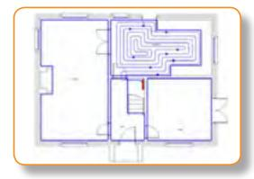
**STEP 3.** To complete the loop, return pipe inside the exisiting pattern back to the manifold maintaining the pipe spacing (typically 200mm).
