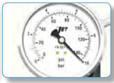
**STEP 5.** If all is well, increase the pressure to 10 bar and leave for a further 10 minutes while checking for leaks or pressure drops.
