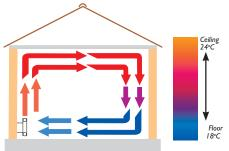
By contrast, radiators transfer heat from a relatively small area at a much higher temperature than the space being heated.
