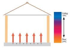
The heat is concentrated where it is most needed for comfort and efficiency.
