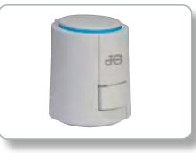
Blue disk in actuator will rise to show valve is open. The actuator comes partly open from factory to assist with initial assembly. On a room by room basis, ensure that all actuators are controlled by the correct thermostat and that each one switches the system on and off. This should also include the boiler being switched on and off.
