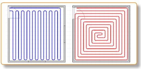
**Diagram 1** - Serpentine is a simple up & down circuit pattern. It is especially good to use when you have irregular shaped rooms or small areas such as kitchens and utility rooms.
