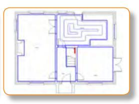
**STEP 2.** Working from left to right or right to left, install first loop working into the centre of the room.
